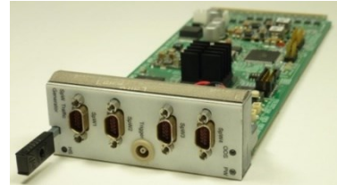
Fig.12.SpW Traffic Generator front view
