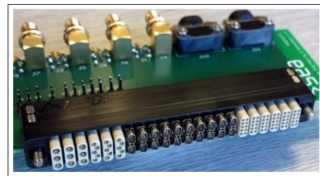
Fig. 2. SpaceWire backplane connector pins
