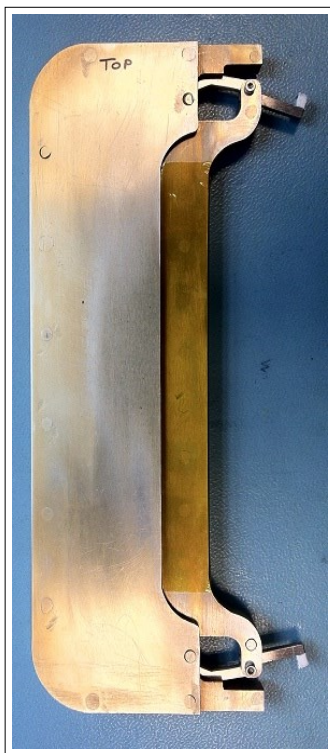
Fig. 10. Extraction tool designed and used by TASUK on Spacecraft units
