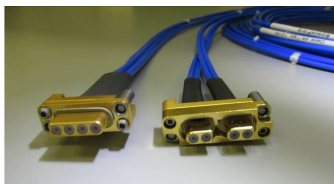
Fig. 1: Left: Reduced size SpaceFibre Demonstrator connector; Right: Existing 2 channel AXOMACH connector
