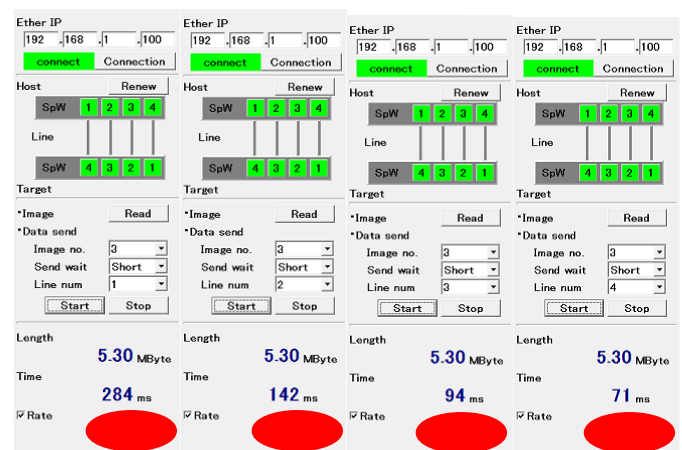
Fig.2. SpaceWire transfer speed
